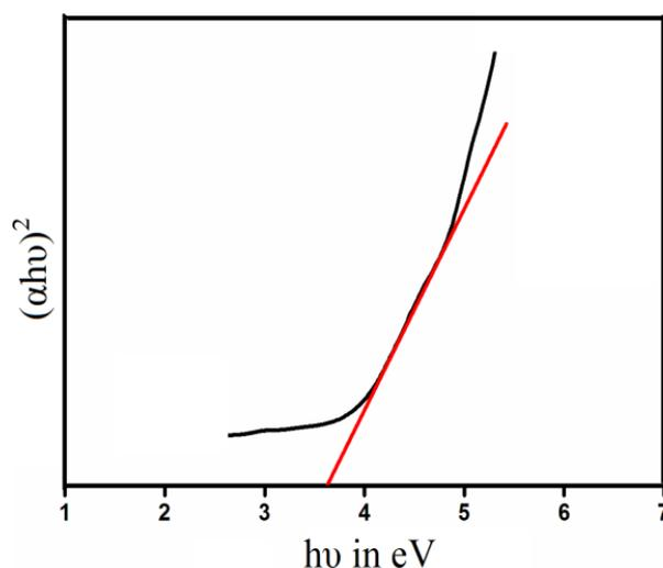
**Fig 3. UV Bandgap energy of  $V_2O_5$  nanoparticles**
