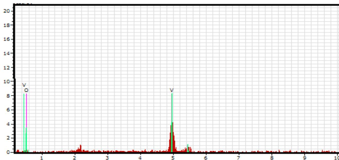
**Fig 5. EDAX spectrum of  $V_2O_5$  nanoparticles at 400°C**
