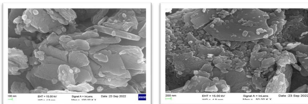
**Fig 4. FESEM images of  $V_2O_5$  nanoparticles at 400°C**
