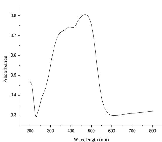
**Fig 2. UV-Vis Absorbance Spectroscopy of  $V_2O_5$  nanoparticles**
