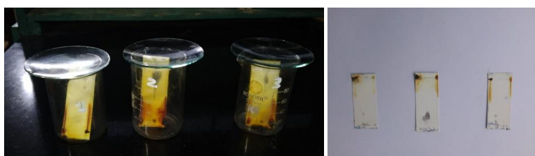
Fig.8 Thin Layer Chromatography images of chlorpheniramine maleate and chlorpheniramine maleate: \alpha -CD in the ratio of 1:1 chloroform: water, ethyl acetate: water
