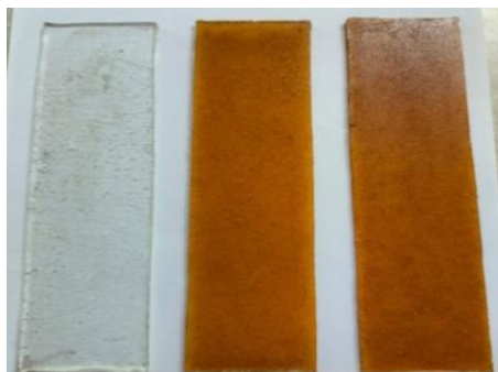
Fig.1: Photograph of the pure and orange peel-imposed epoxy composites
